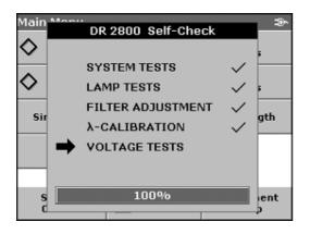
Each time the instrument is powered up, a series of diagnostic tests are performed automatically to ensure operation of major system components.
